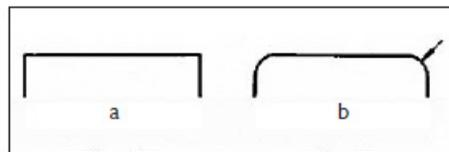
Fig 2 Avoid corners and sharp edges, round off inside edges and penetrations: a) unfavorable, b) favorable.
